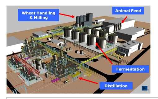
No.1 Ethanol producer in UK, 2<sup>nd</sup> Largest plant in EU 5<sup>th</sup> Largest Biofuel company in EU
